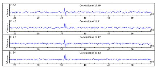
Figure 2 Example of multiple traces in DPA which reveal the key bits of an RSA secret key
