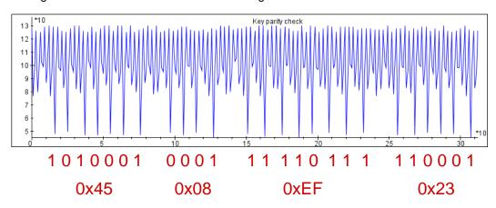
Figure 5: Power trace<sup>1</sup> of a vulnerable key parity check
