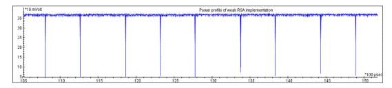
Figure 1: Example of a trace measured during an RSA execution
